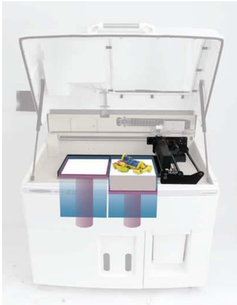
Slika 3. Shema 3D printera, Z510 (ZCorporation, 2005)
